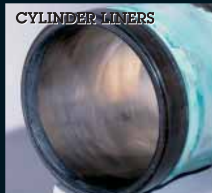
“Probably 95 percent of the crosshatching is still in the liners. No scuffing, no cavitation in the liners. The liners could go back in the condition they’re in.”
