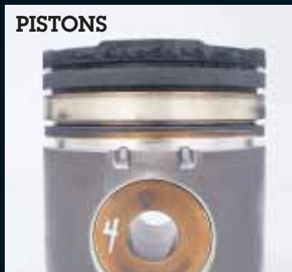
“The pins show no wear at all. The piston crowns and lands show a normal amount of carbon. The skirts are very clean with a few fine vertical lines.”
